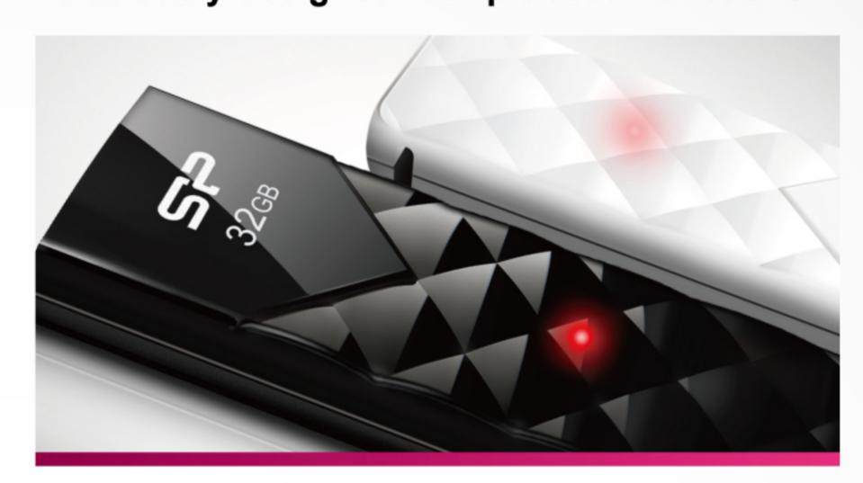
Ultima U03 allows users to carry data around in fashion and ease. It's builts in internal LED indicator illuminates through the front cover to display data transfer status during use.
