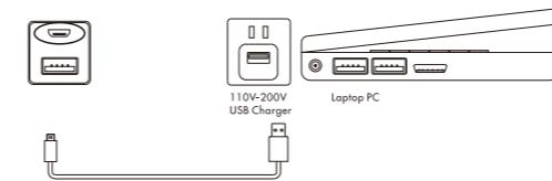
We recommend charging the powerbank 100% before every use. To charge the powerbank, connect the Micro USB connector into the powerbank input port, and the other end to a USB charger or a port on laptop or desktop PC.
